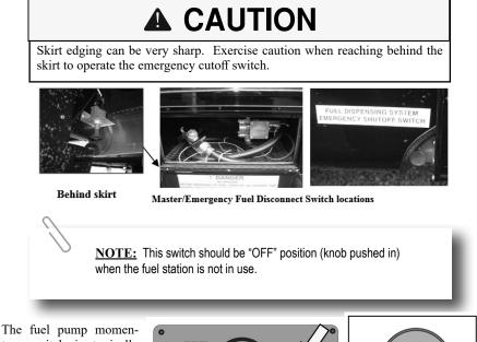
tary switch is typically located inside the RV on the command center panel next to the entrance door (location may vary by model).
