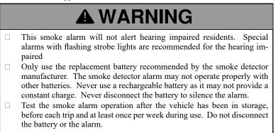
The smoke alarm is operational once the battery is correctly installed. It will not function if the battery is missing, disconnected, dead, the wrong type or not installed correctly. It requires one standard 9V battery. Refer to the user's guide, for correct battery and installation information,
